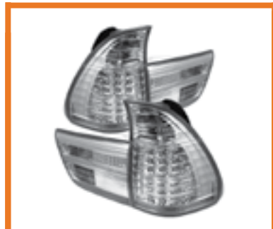
BMW E53 X5 00-06 4-PC LED Tail Lights - Chrome PART#: ALT-YD-BE5300-LED-C SKU#: 5000798 UPC#: 847245000798
